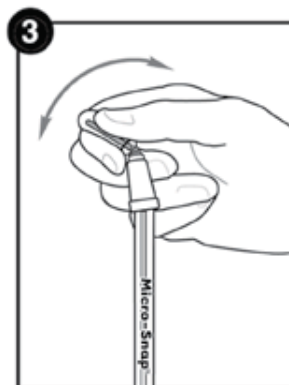
3. Activate device by breaking the snap valve with a snap and squeeze action.
