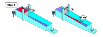
**Step 5** - Look at how far the product ran down the slope in the 30 sec. The slope has graduation marks indicating the distance in centimeters. Record this value as the consistency of the product.
