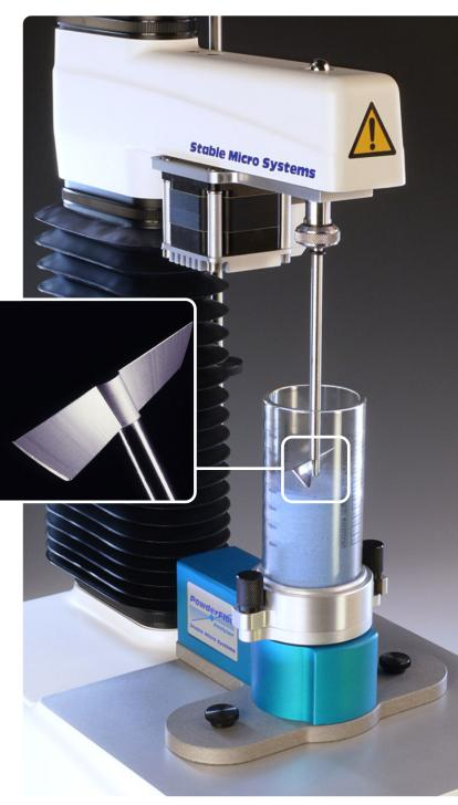
The Powder Flow Analyser unit may be attached to or removed from the TA.XTplus Texture Analyser within minutes
